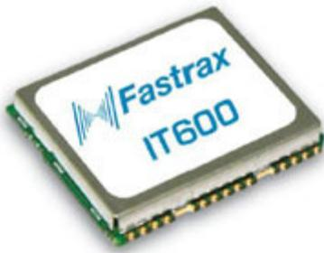
Advanced dead reckoning estimates the position of the vehicle when satellite signals are unavailable – which inevitably happens in tunnels and parking garages. The IT600 can utilize an analog gyro and odometer pulse and can later be complemented with a digital 3-axis gyro and differential wheel pulse from a vehicle's CAN interface in order to compensate for possible unavailability of GNSS signals.
