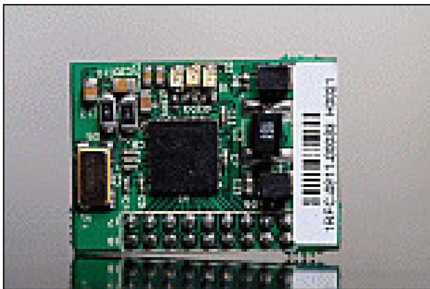
Yitran, available through [GLYN High-Tech Distribution](#), releases the IT700, a highly integrated System-on-a-Chip (SoC) Powerline Communication (PLC) IC that incorporates Yitran's extremely robust Physical Layer (PHY), high-performance Data Link Layer (DLL) and Network (Y-Net) protocol. IT700 also features a 8051 Micro with 256 KB Flash for protocol stack and application implementation as well as 24 general purpose I/Os.
