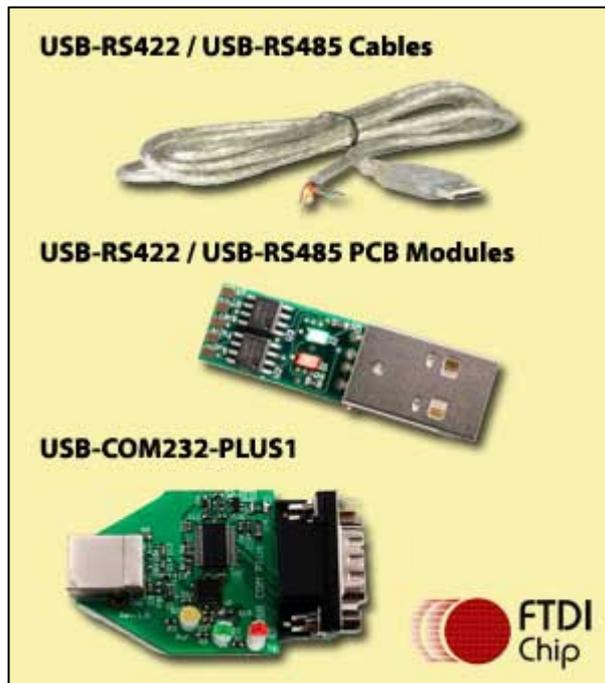
Future Technology Devices International (FTDI) announced recently the availability of two serial interface converter cables that incorporate transceivers to facilitate connecting RS-422 or RS-485 based peripherals to a PC's USB port. Using FTDI's FT232RQ USB to asynchronous serial interface IC, the USB-RS485-WE converter cable includes an RS-485 transceiver while the USB-RS422-WE cable utilises a RS-422 transceiver. The far end of the 1.8m cables are wire ended (no connector).
