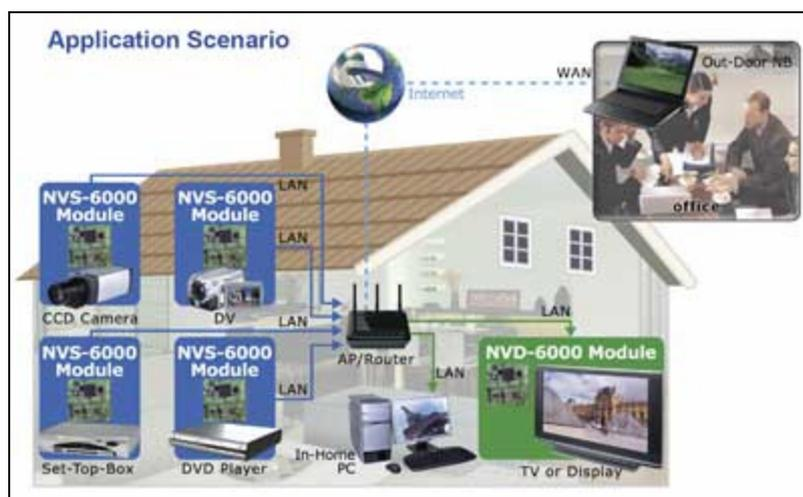
NVS-6000 compresses NTSC/PAL video signal with different resolutions (Full-D1 max.) into H.264 Baseline/Main profile stream. It also provides different audio stream formats whenever the audio compression algorithm is used.
