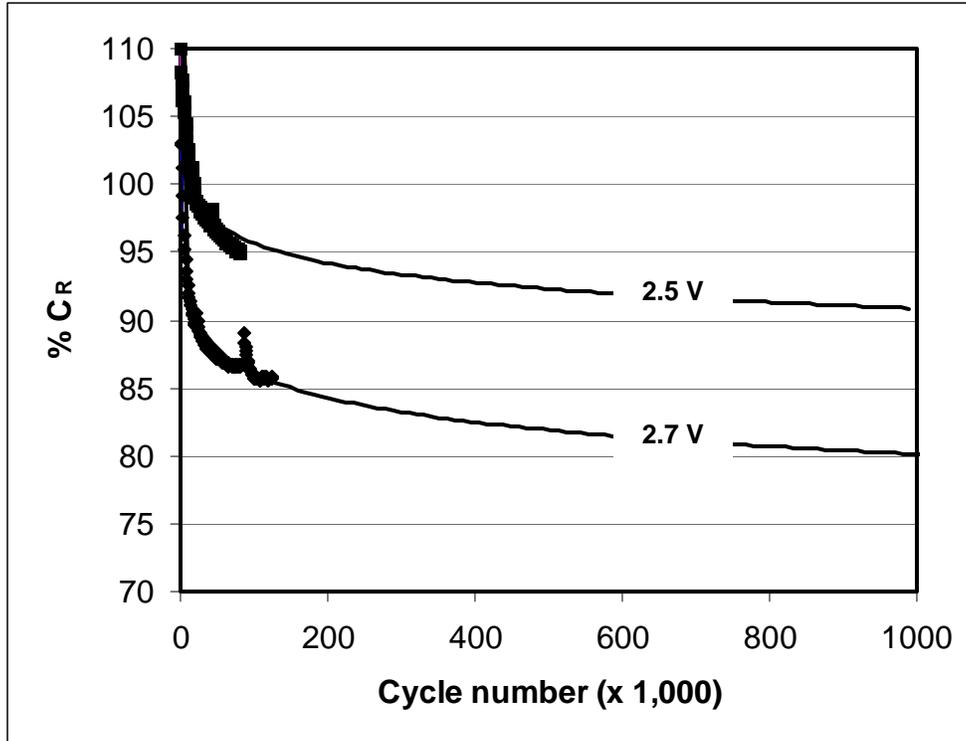
Figure 6: Capacitance change vs. continuous cycling
