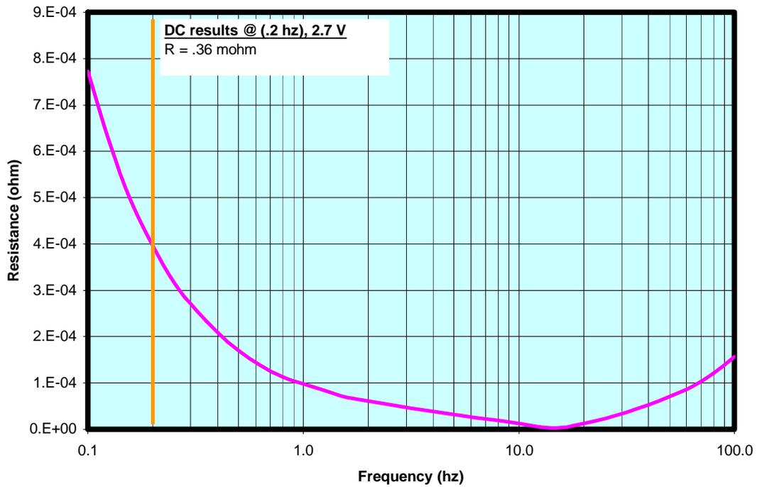
Figure 15: BCAP2600-E Resistance Frequency Response
