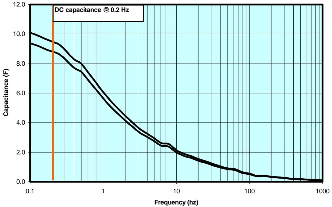
Figure 10: PC10 Capacitance vs. Frequency Response, 95% Confidence
