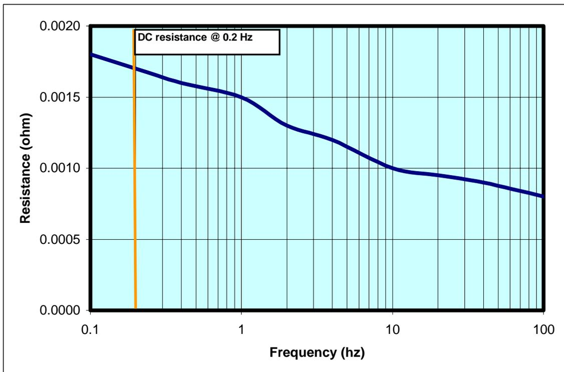
Figure 13: BCAP0350-E Resistance Frequency Response
