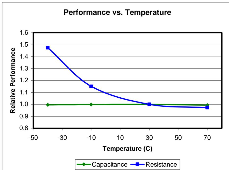
Figure 3: Relative ultracapacitor performance over operating temperature range
