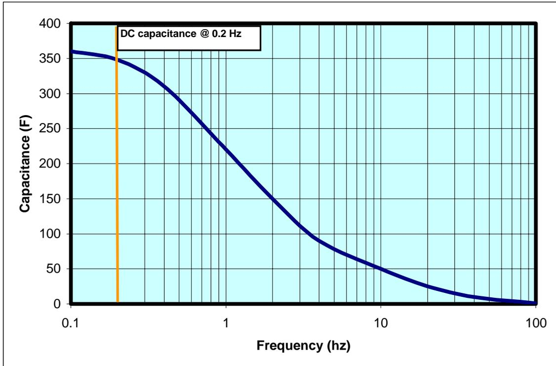
Figure 12: BCAP0350-E Capacitance Frequency Response
