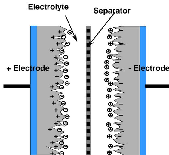
Figure 1: Ultracapacitor charge separation
