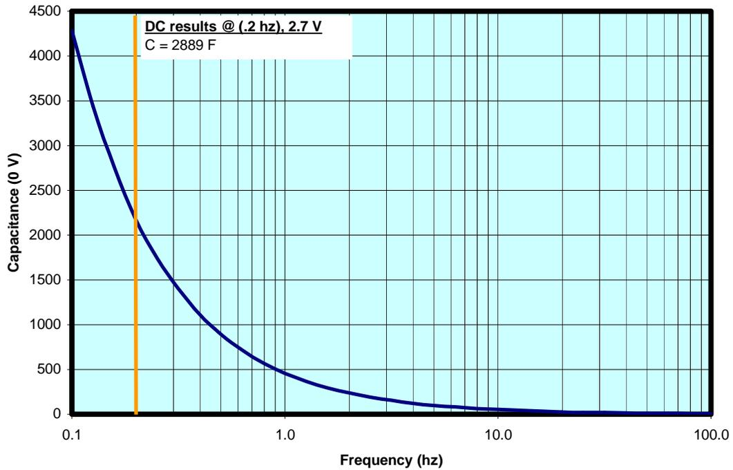
Figure 14: BCAP2600-E Capacitance Frequency Response
