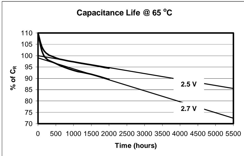
Figure 4: BCAP2600 Capacitance degradation at 2.7 V and 2.5 V at 65°C
